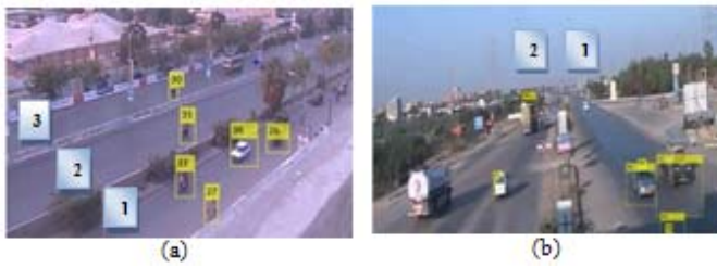
Fig. 3. Detection results obtained from Blob Analysis. Lanes are labeled as 1, 2 and 3 (a) NIPA (b) TOLL PLAZA Datasets
